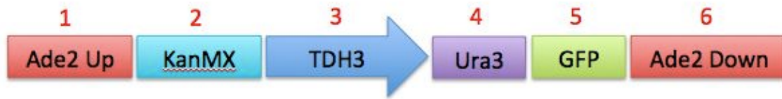
Figure 1. Construct created by BrickMason assembly. It is composed of 6 parts, the parts will be referred to by the red numbers shown above them.
