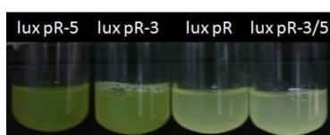
The strength of *lux pR* promoters were characterized by measuring the fluorescence of *E. coli* cells with IR-GFP
